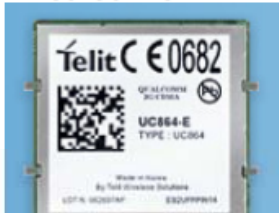
Small low cost modems 30x36x4.8Xmm
